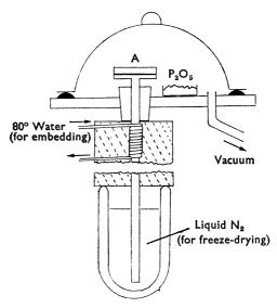
The apparatus is also suitable for the vacuum embedding of treated tissue. A coil of copper tubing surrounds the rod immediately below the bung. When water at 80° C is circulated, sufficient heat is conducted to melt embedding wax in the tissue holder.
